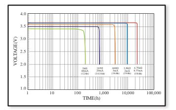
1. Typical discharge profile at  $+20^{\circ}$ C (Typical value)
